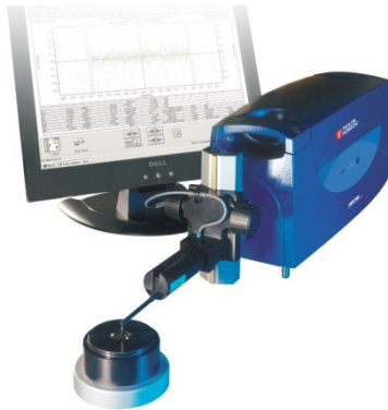
Fig. 1. Measuring equipment Taylor Hobson Talysurf Intra 50
